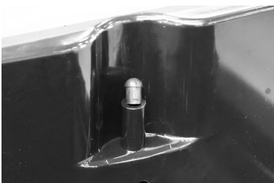
3. Remove the sealing nipple from the front drain plug of the TTK 200 and plug it onto the lower drain opening to seal this drain. Now plug the fabric hose onto the front drain plug.
