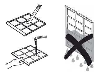
3. Allow the filter to dry completely. Do not insert a wet filter into the device!
