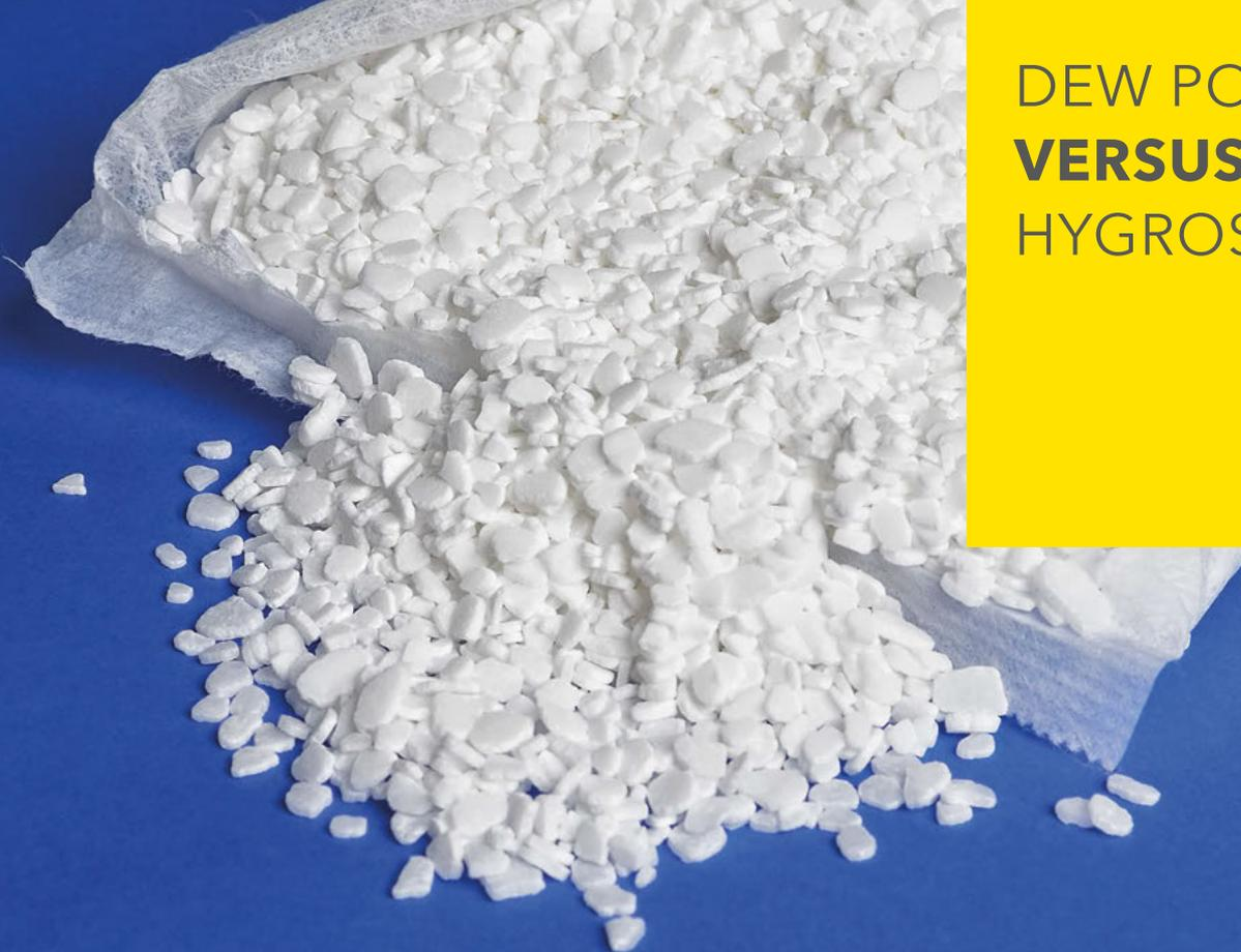
The figure above shows the content of a typical refill pouch for passive dehumidification by means of granules. These disposable pouches usually contain highly hygroscopic salts such as calcium chloride serving as a drying agent that can withdraw moisture from the room air by desiccation.
